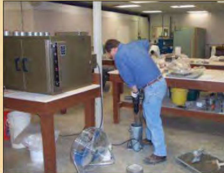
Fabricating cylinders with vibrating hammer (ASTM C1435)
